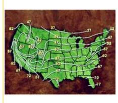
At a depth of below four feet, the ground temperature stays a constant 50 to 55 degrees year-round.
