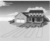
Horizontal closed loop installations are generally most cost-effective for small installations, particularly for new construction where sufficient land area is available. These installations involve burying pipe in trenches dug with back-hoes or chain trenchers. Up to six pipes, usually in parallel connections, are buried in each trench, with minimum separations of a foot between pipes and ten to fifteen feet between trenches.
