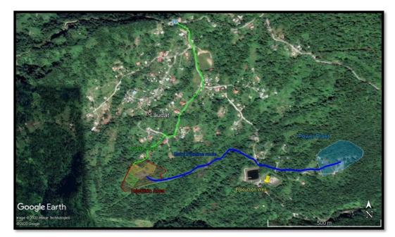
Figure 4: Location of Proposed Geothermal Plant, Reinjection Pipeline, Well & Access Road
