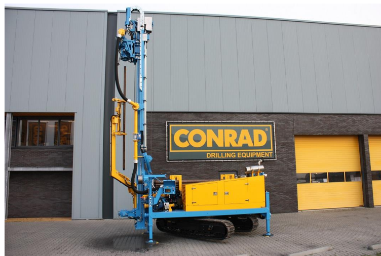
Figure 47. Typical drilling rig for shallow geothermal drilling (Conrad Boxer 200)
