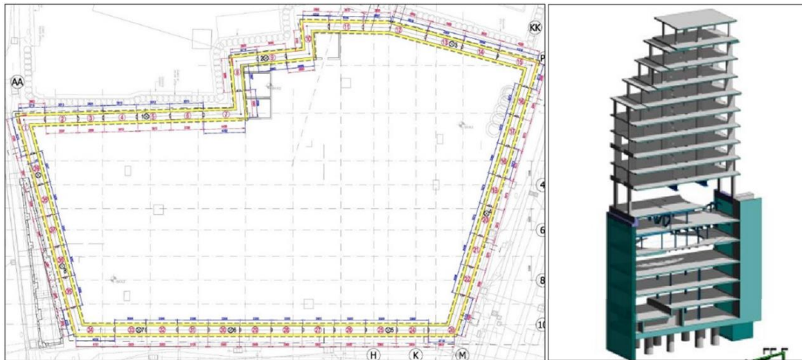
Figure 58. Diaphragm Wall panel layout (left) and 3D section of superstructure and basement (Source: Amis, T et al. Integrating geothermal loops into the diaphragm walls of the Knightsbridge palace hotel project)
