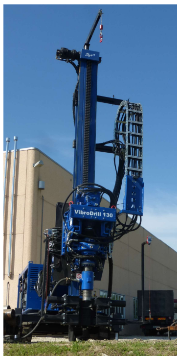
Figure 7: Drilling machine with roto-vibrating drill head (photo Hydra srl)
